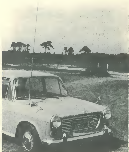
The neat appearance of the 160 metre whip when mounted in position
