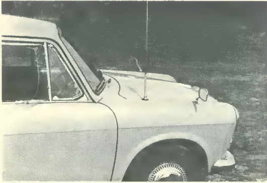
The whip aerial mounted on the existing car aerial
